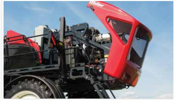
Engine and hydraulic service checkpoints are easy to access from the walkway by the engine compartment.
