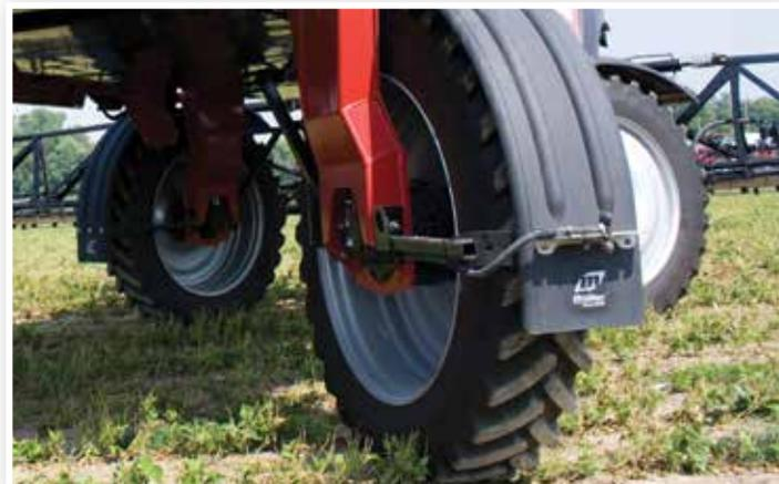
With the 4-wheel steer option, you'll have the tightest turning radius in the business. With front and rear wheels following the same track, crop damage is minimized and headland turning is a snap.
